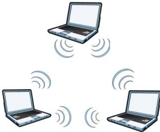
Figure 625 Peer-to-Peer Communication in an Ad-hoc Network
