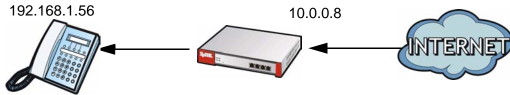
Figure 99 WAN to LAN H.323 Peer-to-peer Calls Example
